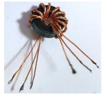
Now use a DVM to test for continuity. Re-arrange the wires so that there is continuity from A-A, B-B, and C-C in this photo.
