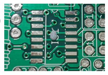
Check the pins of the FST3253 and if any are bent, straighten them carefully and very gently. Place the IC on the PCB with the small dimple aligned with the mark on the PCB. It is very important to orientate this IC correctly. You can check the alignment of each pin against its PCB pad using a jeweller's loupe or magnifying glass. (below left).
