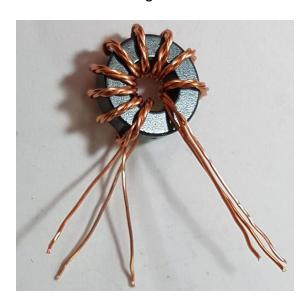
Now it's necessary to identify which wire belongs to which winding. You have three windings twisted together, they all use the same wire. The only way to do this is with a DVM as continuity tester. First, untwist and straighten the wire ends that are not wound around the toroidal core.
