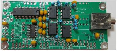
Note that only a very little solder is required. The solder will tend to fall through the hole to the other side of the PCB. So too much solder, will cause a big blob on the other side of the PCB that could cause shorts etc. Therefore only a little solder, soldered quickly with the soldering iron tip, is generally enough.
