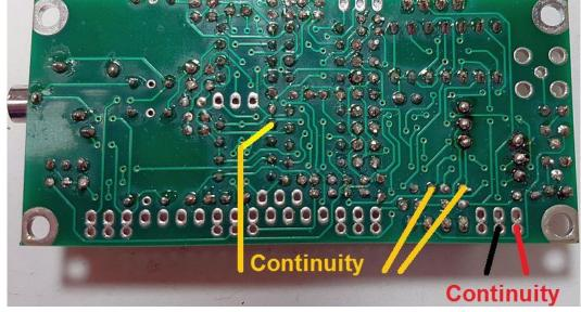
ends of the two 82-ohm resistors R26 and R27. Hold the black probe on IC6 pin 1. Hold the red probe on the resistor ends as indicated by the two nearby orange lines.
