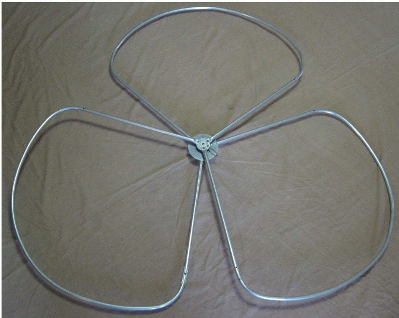
Photo 1 146MHz 3 Petal Cloverleaf assembled.
