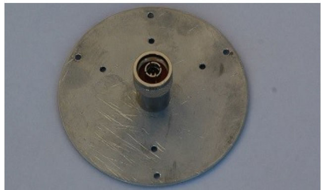
Photo 3 3 Petal Cloverleaf lower hub plate assembled.
